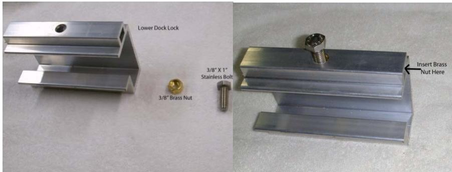
8. Place 2 dock locks on the bottom rail of dock #1. Then add dock #2 into the dock locks. The fit should be tight. Make sure the tops of each dock are level with each other. Tighten bolt to 10-15 ft/lb. DO NOT OVERTIGHTEN.
