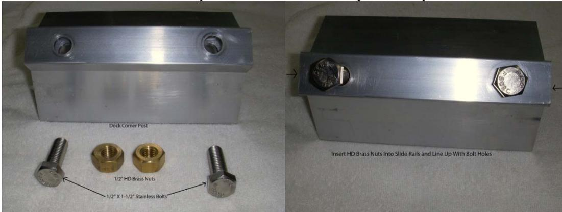
4. Slide post into corner pocket to estimated length for your water depth. Tighten bolts to 10-15 ft/lb. DO NOT OVERTIGHTEN.
